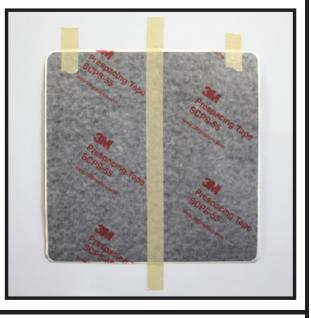
3. Lift the graphic away from the vehicle and gently separate the paper liner from the film all the way to the hinge. At the hinge make a straight cut across the liner, using care not to scratch the vehicle or damage the part.
